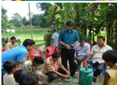
Photo 21: Demonstration of treatment process by boucheri
