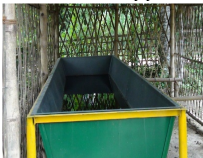
Photo 20: Bamboo treatment tank machine treated bamboos
